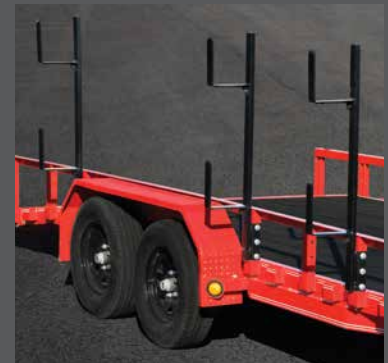
PIPE UTILITY RACK
