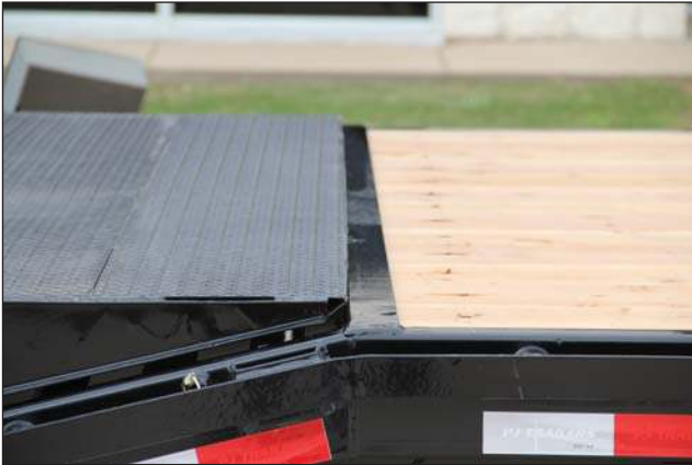
Tail Folded Flat for Storing Cargo
