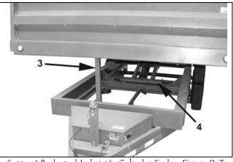
Support Body and Lubricate Cylinder Ends - Figure 8-3
